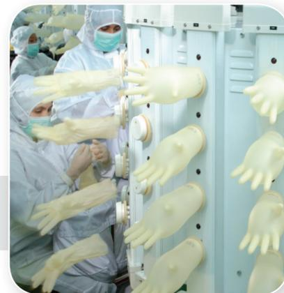
Every Biogel glove is 100% air inflation tested and visually inspected for holes<sup>8</sup>
